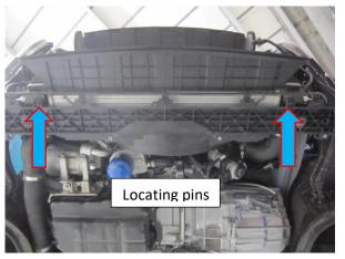
**11**. To remove the OE intercooler, first undo the two hose clamps securing the boost hoses to the intercooler. You will need an 8mm socket and rachet drive or a flat blade screw driver to loosen them off
